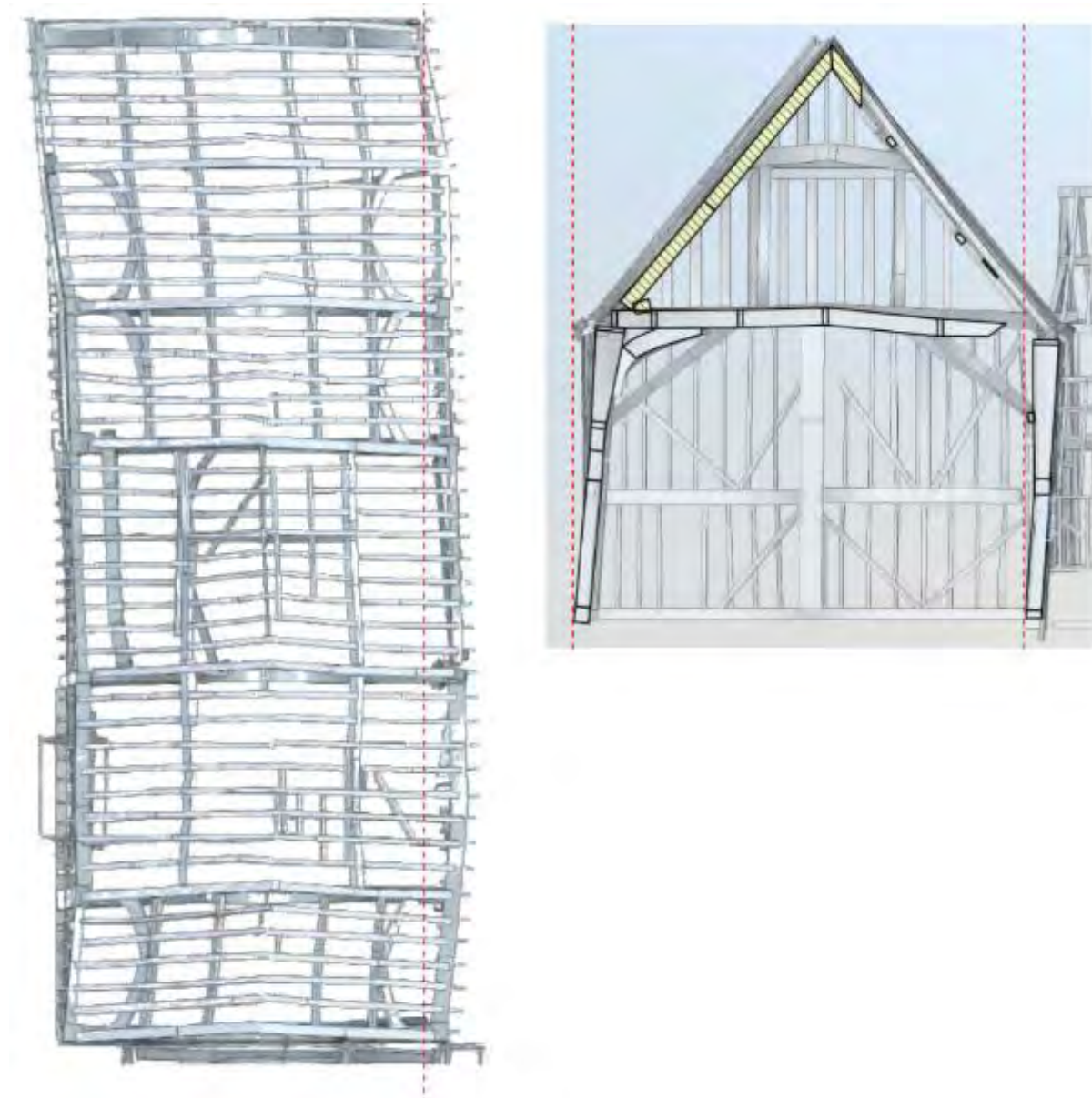
Figure 2: Extract from digital model showing extent of visible racking within frame
